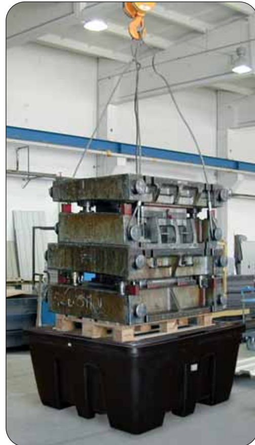
PE-KT-1S under a test load of 8.000 kg
