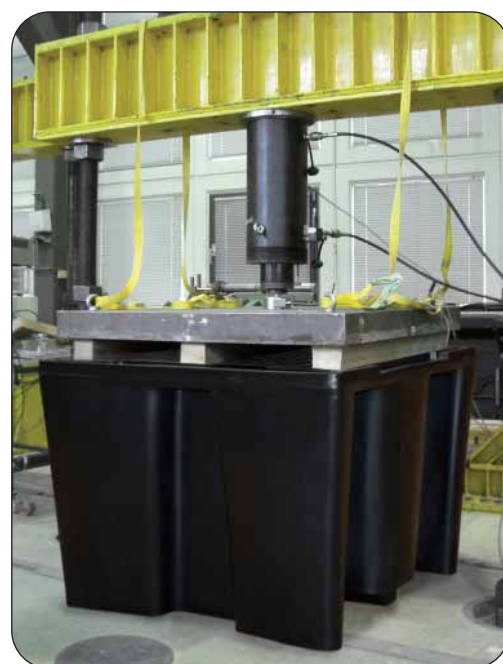
PE-KT-1 under a test load of 8.000 kg
