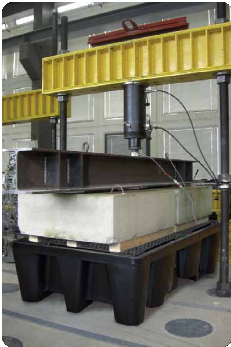
PE-KT-2 under a test load of 16.000 kg
