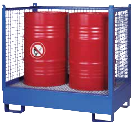
Model WSP-25SS WSP-25KS/Gitt WSP-45KS/Gitt Capacity, 200 liter drums 2 2 4 External dimensions W x D (mm) 1410 x 810 1410 x 810 1410 x 1290 Total height (mm) 1300 1410 1320 Internal dimensions W x D (mm) 1320 x 720 1320 x 720 1320 x 1200 Compartment height (mm) 950 1025 1025 Sump capacity (l) 220 220 220 Max. load (kg) 500 500 1000 Article no., painted P21-2451-A P21-2510-A P21-2510-A Article no., fire-galvanized P21-1451-A P21-1501-A P21-1510-A
