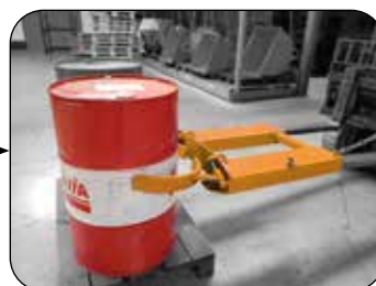
FG 2216/1, RAL 2004 - pure orange, Article no. B69-6356-A, L x W x H (mm): 1285 x 710 x 150, Load capacity: 400 kg
