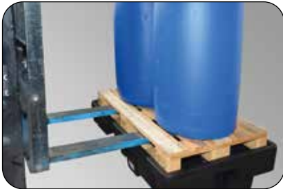
Safe positioning of the Euro pallet
