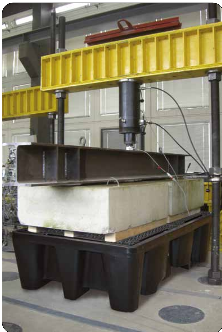
PE-KT-2 under a test load of 16.000 kg
