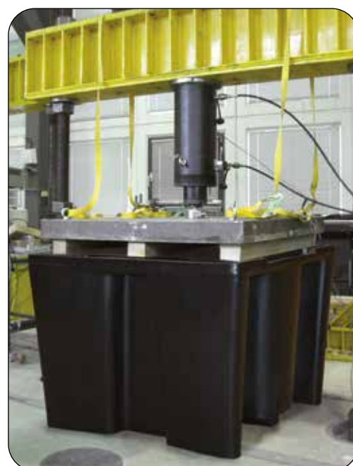
PE-KT-1 under a test load of 8.000 kg
