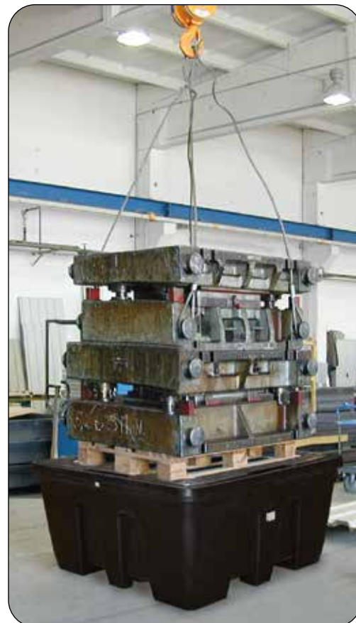
PE-KT-15 under a test load of 8.000 kg
