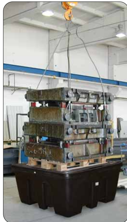
PE-KT-15 under a test load of 8.000 kg
