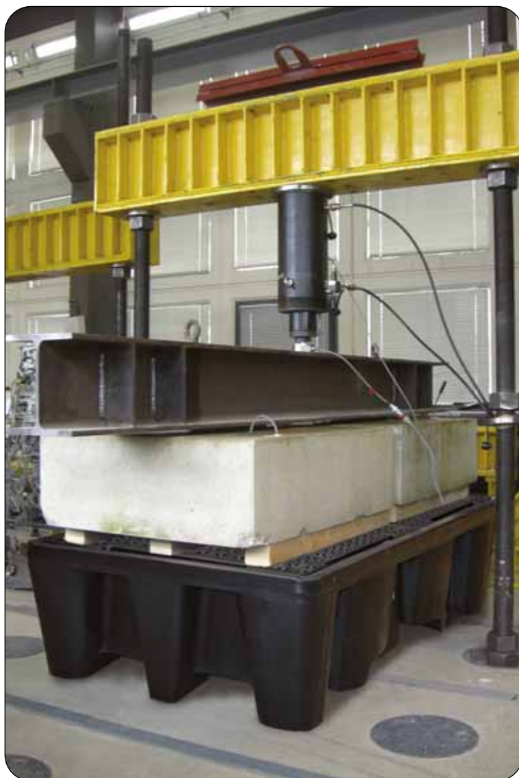
PE-KT-2 under a test load of 16.000 kg
