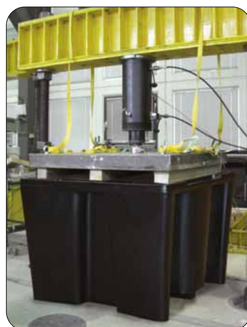
PE-KT-1 under a test load of 8.000 kg
