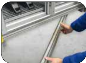
Cabinet accessible with lift truck thanks removable socle panel
